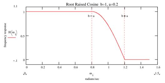
These two graphs should make the difference obvious. The RRC function has a sharp corner at the upper edge of its transition band. And one can see how the flat parts are connected with a piece of cosine. The RRC uses 90 degrees worth and the RC uses 180 degrees worth of cosine.
