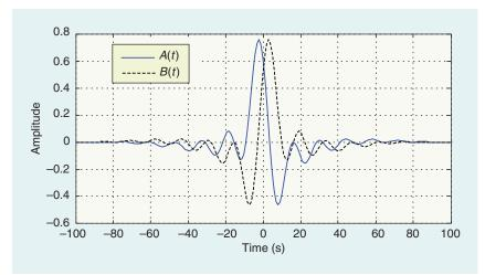
[FIG4] Rotated (±45°) filters' impulse responses.
