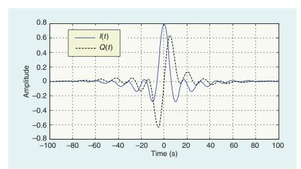
[FIG3] In-phase and quadrature phase filter impulse responses.
