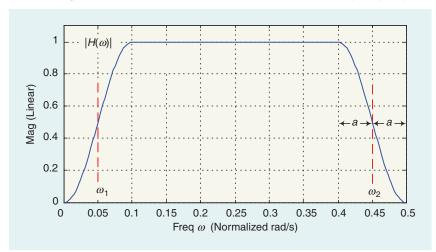
[FIG2] Desired analytic signal generation filters' magnitude response.
