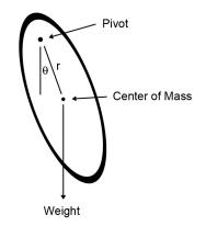
In this diagram, the pendulum has a mass, *m*, and the center of mass is displaced from the pivot by a distance *r*. The pendulum's angular displacement is  $\theta$ . To find the equation of motion,  $\theta(t)$ , let's 1<sup>st</sup> review torque. If a force, *f*, acts on a lever arm of length, *r*, at an angle of  $\theta$ , the torque,  $\tau$ , will be
